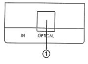
**1. TOSLink (Optical Fiber) Input Port:** Connect the TOSLink input port to the TOSLink output port of audio equipment such as audio amplifier, AV receiver or DVD player.
