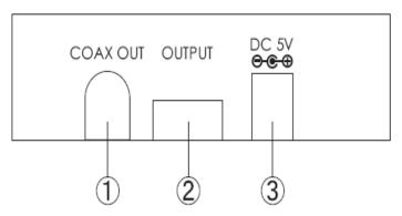
①. **COAX OUT:** This slot is where you connect an amplifier for transmitting an audio signal with coaxial cables. When the audio return function is on the audio signal will be received from the output and when the audio return function is off the audio signal will be received from the input source.
