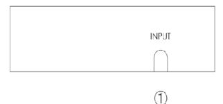
① INPUT switch: Press the button repeatedly to switch to your desired input source.
