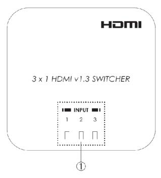
① Input LED indicators: Press the INPUT button repeatedly to switch to your desired source and the LED will turn on to indicate which input source has been selected.
