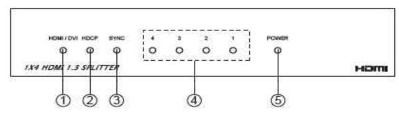
**1 HDMI/DVI Indicator:** The LED will illuminate when the selected HDMI input source is originally from an HDMI output, the LED will illuminate when the selected HDMI input source is originally from a DVI output.
