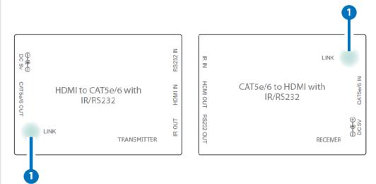
**1. LINK LED:** This LED will illuminate in blue when the devices are connected with a CAT5e/6 cable. If the data transmission has an error the LED will blink
