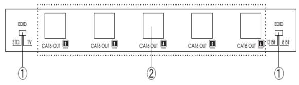
① **EDID Control Switcher:** Switch the EDID between STD & TV. Switch to STD to use the built-in EDID or switch to TV to use the TV's EDID. Default factory setting is on TV, leave as is when the display is working properly. By switching
