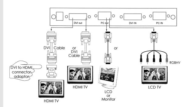
The DVI Digital scaler with ultra high bandwidth can output a variety of PC, SD and HD resolutions in both digital and analog format simultaneously.
