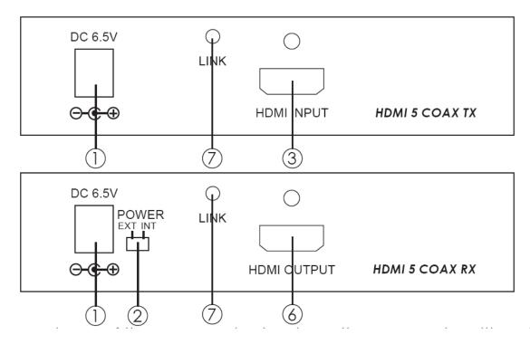
1 Connect one of the power adaptors to Active Connect multimedia Transmitter Box and plug in the power. May also plug the other adaptor to Active Connect Multimedia Receiver Box.
