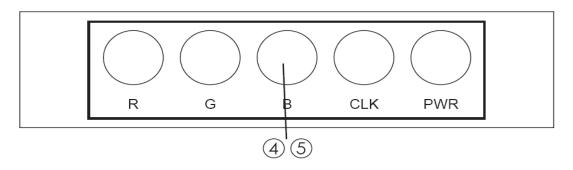
4 Connect BNC-F connectors to both sides of the 5 cables.
